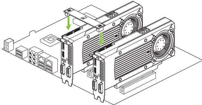
If you are installing a third GeForce GTX 660 Ti graphics card for a 3-way SLI configuration, continue with step 7. Otherwise, go to step 8
