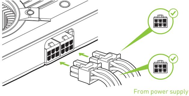
If your power supply needs an additional 6-pin power connector, you can use the included 4-to-6 pin adapter. Make sure to connect each 4-pin connector to a separate PSU cable.
